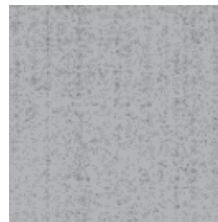
Fig. 3 Simulated image using a friction noise function at 100% image density. For better visualization, image contrast has been enhanced and positive/negative has been reversed. Thus, the dark areas indicate removed toner.
